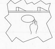
Step 5 Carefully tighten the four mounting screws. The mounting wings will secure the speaker in place.
