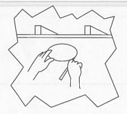
Step 4 Attach loudspeaker wires to speaker terminats, position speaker frame up into cutout.
